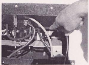
13. Attach negative lead to B negative on speed control, and touch front terminal to black or brown cillinoid. Voltage should read 45 to 52 Volts.
