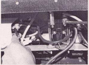
14. Move hot lead to forward-reverse cillinoid on blue wire. Should read 45 to 52 volts.
