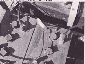
12. Check the red wire opposite the on and off cillinoid in line fuse. This should read 48 volts.
