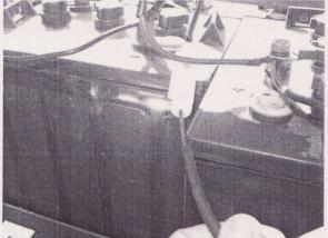
20. With the negative lead still on B negative, back probe the red wire with a white stripe on the speed control where the white malox plug is. This should read 45 to 52 volts.
